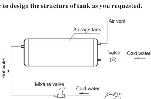
1. Connect pipes as above suggested. Make sure no leakage in pipeline, joints, valves and so on.
